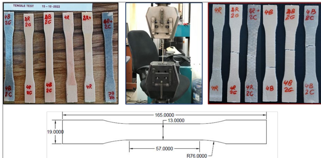
Fig. 2: (a) The samples before tensile testing, (b) Testing apparatus, (c) The samples after tensile testing, and (d) The standard sample dimensions.
