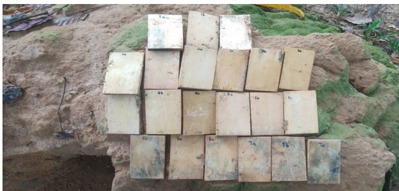
Fig. 6: Rubber wood blocks after being buried in a termite mound for 30 days.
