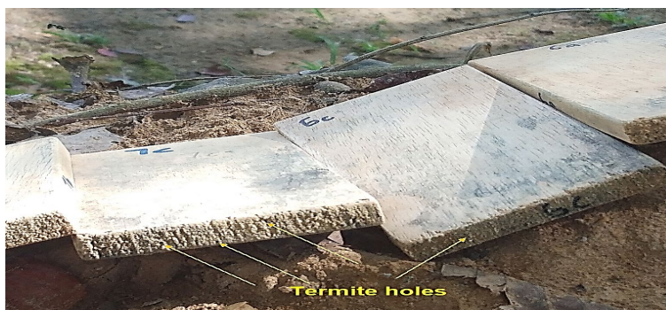
Fig. 5: The effect of termite bite holes on samples No.6 and 7.
