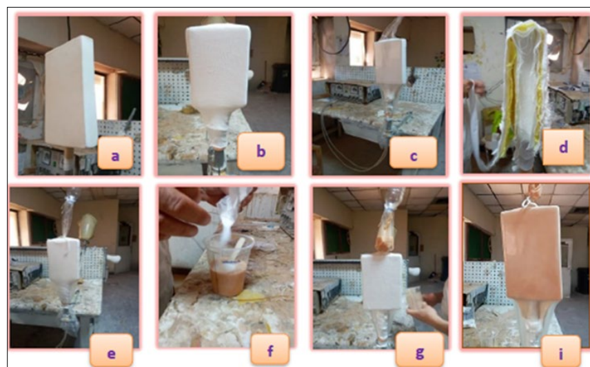
Fig. 1: Demonstrates the process of preparing test specimens for a knee prosthetic socket and depicts the various steps involved in the preparation procedure.
