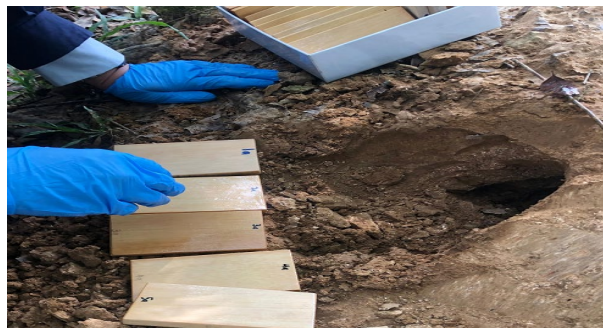
(e) Rubber wood blocks installation into the mound.
