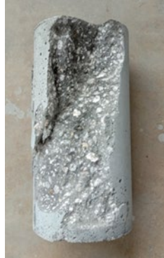
Figure 6. Cracked concrete sample of Adjusted mix design
