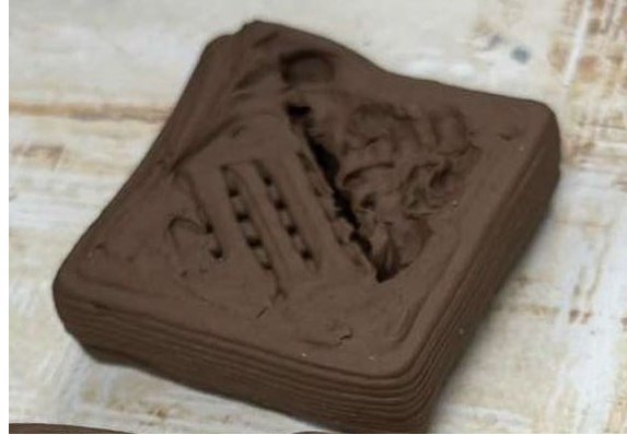
Fig.5 2x2 3D-Printed Sample Showing Non-Uniform Extrusion Due to Air Entrapment and Pressure Backflow.
