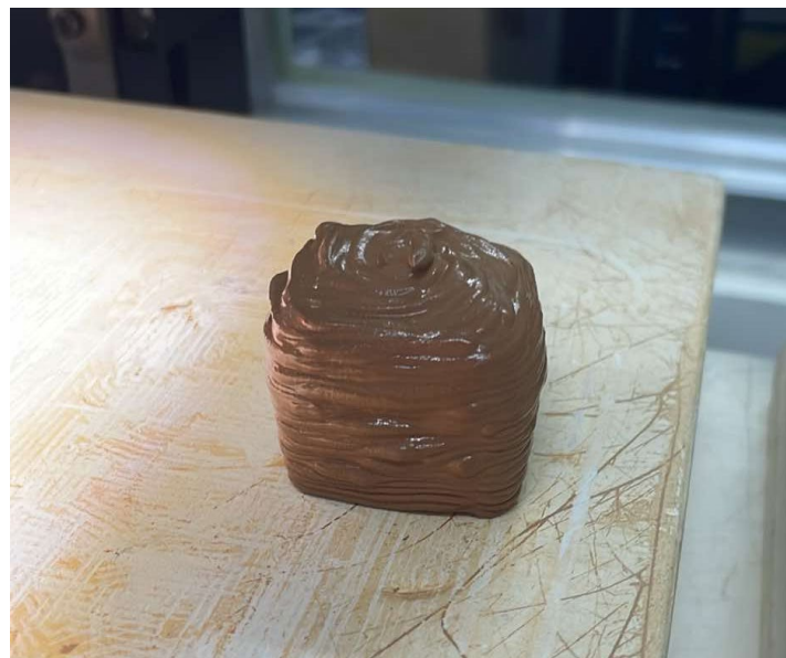
Fig. 4 2x2 3D-Printed Sample Block Print Irregularities due to Excessively Wet Mixture.
