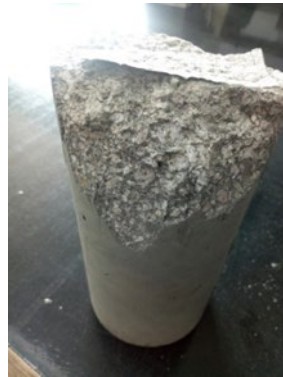
Figure 3. Cracked concrete sample from Compressive test
