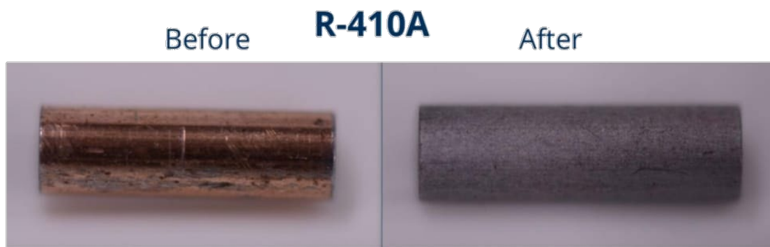
Figure 1: Compatibility test results of a steel material subjected to a nano lubricant-refrigerant mixture.
